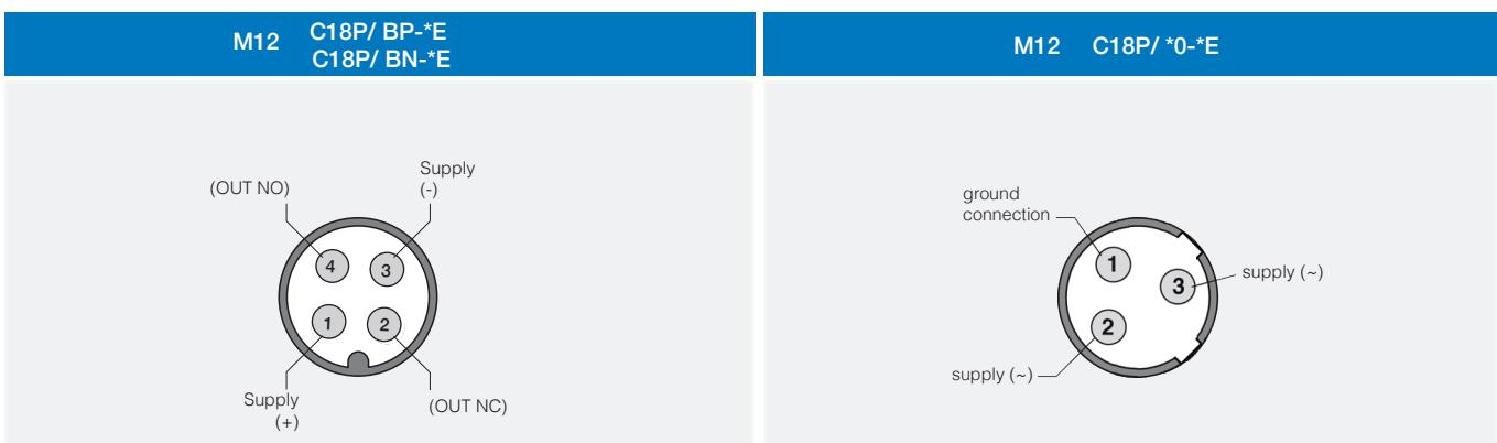
For models with AC power supply using the connection cable series CD12M/AC
