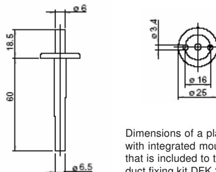
Dimensions of a plastic tube with integrated mounting plate, that is included to the duct fixing kit DFK 200
