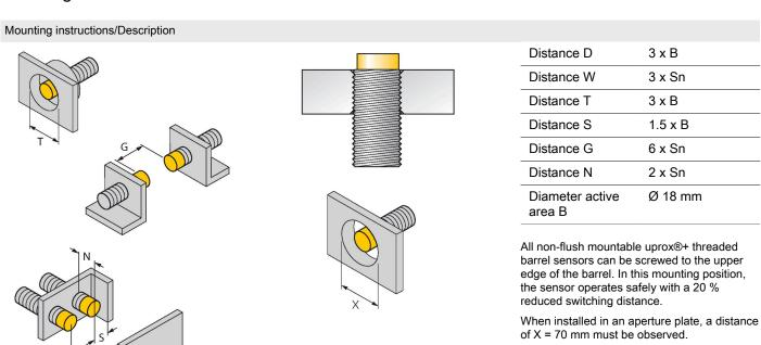
Mounting bracket for threaded barrel sensors; material: Stainless steel A2 1.4301 (AISI 304)
