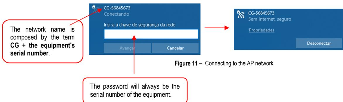
Figure 11 – Connecting to the AP network
