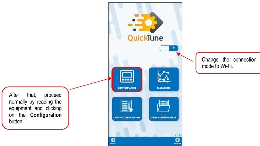
Figure 14 – Wi-Fi connection
