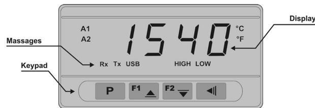
Figure 7 Identification of the front panel parts
