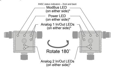
\* Indicator LEDs are visible through translucent housing
