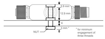
Screw Length (with screw head fitting in counterbore) = 12.9 mm + "X" mm + 3 mm
