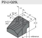
Floating positioning element for linear position sensors LI-Q25L; the nominal distance to the sensor is 1.5 mm; pairing with the linear position sensor at a distance of up to 5 mm or misalignment tolerance of up to 4 mm.
