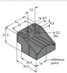
Floating positioning element for Li-Q25L linear position sensors; operational at an offset of 90; nominal distance to sensor 1.5 mm; pairing with linear position sensor at a distance of up to 5 mm; misalignment tolerance of up to 4 mm P6-LI-Q25L
