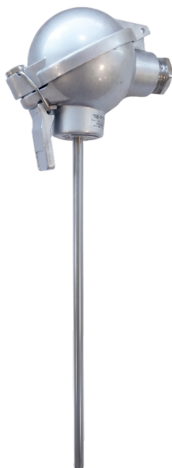
ATI-P1-A-S-6-100-NAA-ON: Pt100 Class A, Ø 6 x 100 mm, mineral-insulated, NAA head IP67
