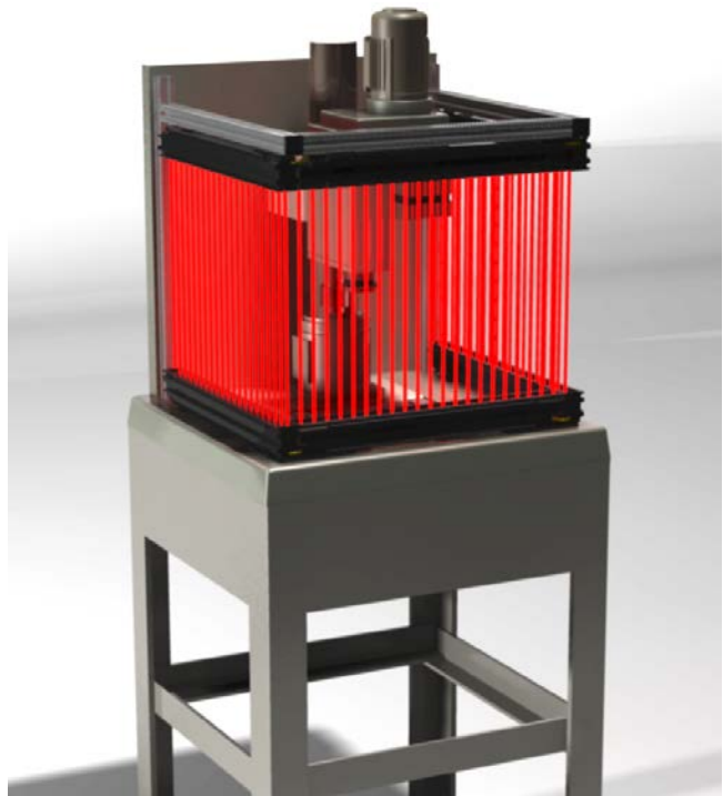
Figure 35. Cascaded light curtains guarding a u-shaped cell
